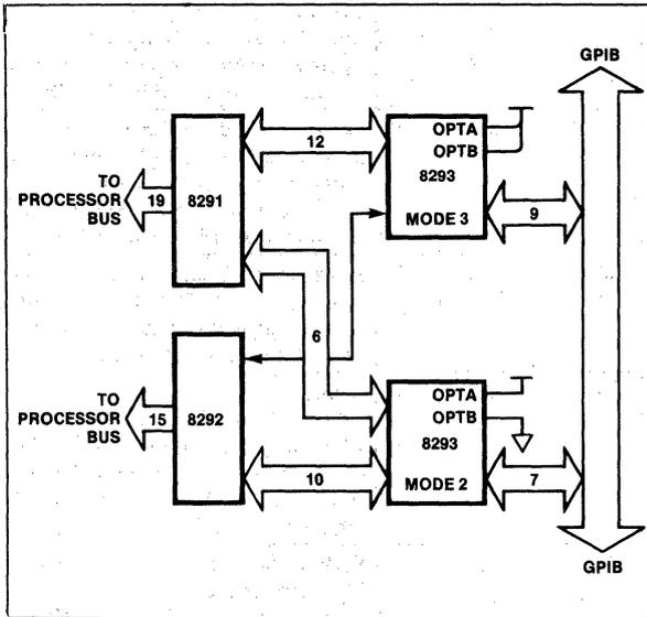
**Figure 3. Talker/Listener/Controller Configuration**
