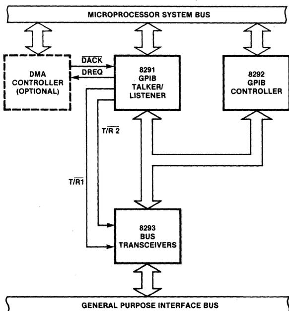
Figure 1. 8291, 8292 Block Diagram
