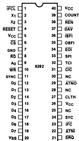
Figure 2. Pin Configuration
