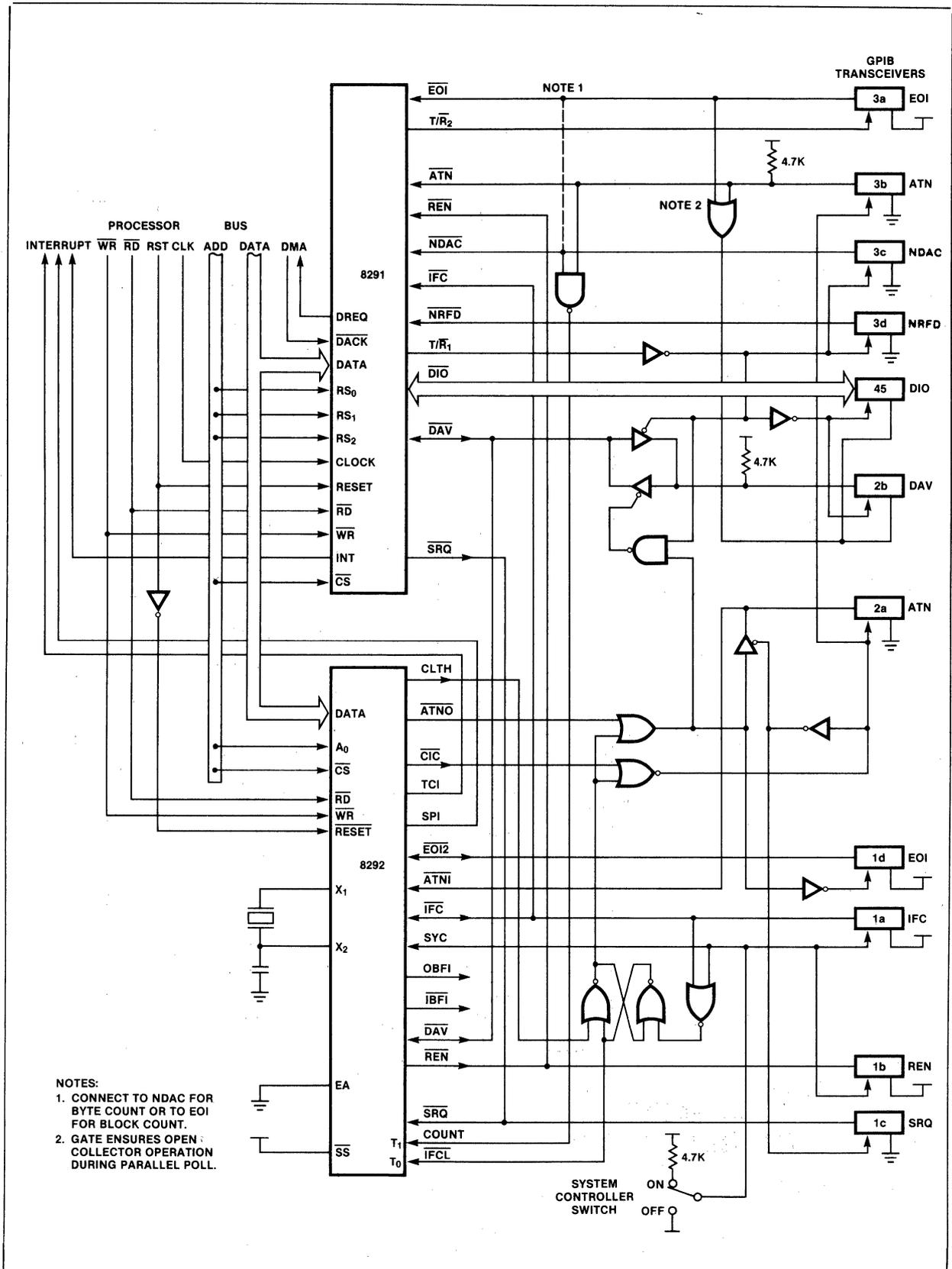
Figure 4. 8291 and 8292 System Configuration
