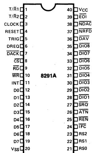
Figure 2. Pin Configuration
