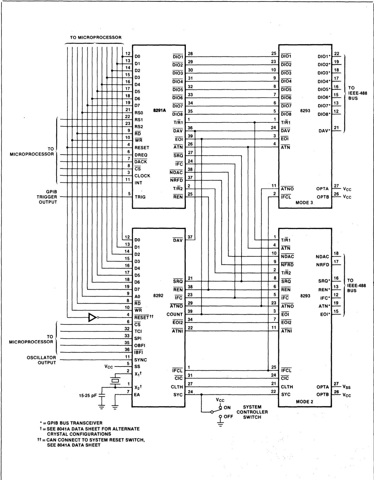
Figure 7. 8291A, 8292, and 8293 System Configuration
