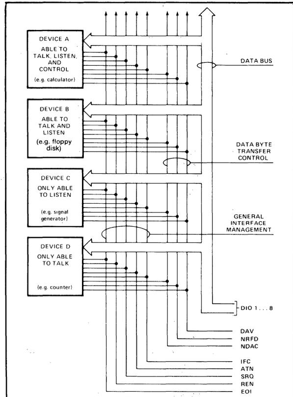
Figure 4. Interface Capabilities and Bus Structure
