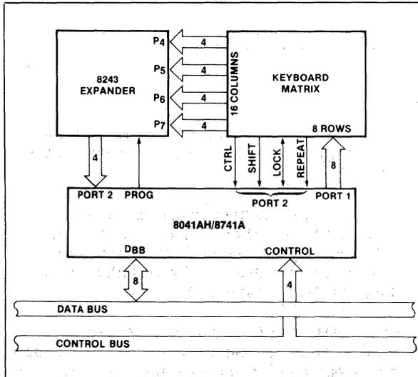
Figure 5. 8041AH-8243 Keyboard Scanner
