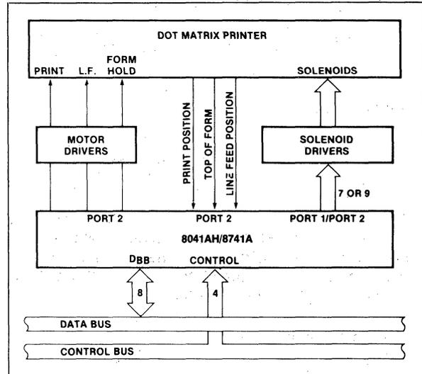
Figure 6. 8041AH Matrix Printer Interface
